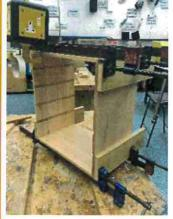
Sand pieces and glue to form box shape - p80, p120, p240, wet and dry paper, sanding block, tape measure, 4 x Sash-Cramps, tri square, scarp wood, PVA
