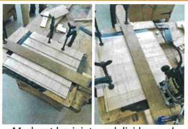
Mark out lap joints and dividers and then cutting with wood router - Tape measure, steel ruler, tri square, sharp pencil
