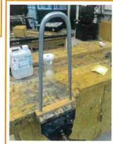
Gluing handle into beech stand - Epoxy resign, vice, scrap wood, smaller piece of long wood (pen like shape)
